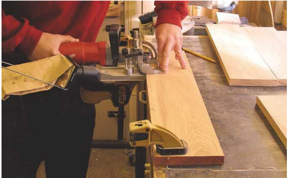
▲ Pic.2 Clamp the boards to the bench, then cut the slots for the biscuits and brush glue into them
